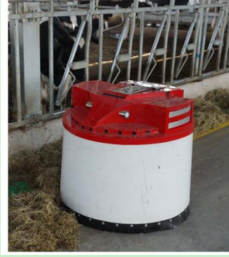
Figure 1. Automated feed pushing robot (Haotun et al., 2018).
