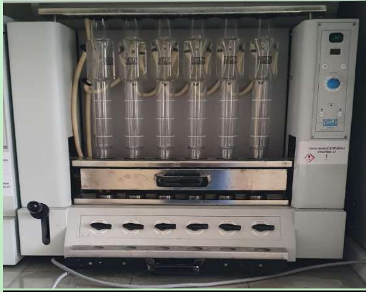
Figure 1. Device used in cellulose determination
